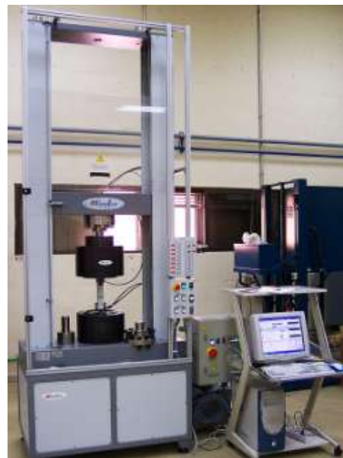
Microtest EM2 Series 500 kN universal testing machine
